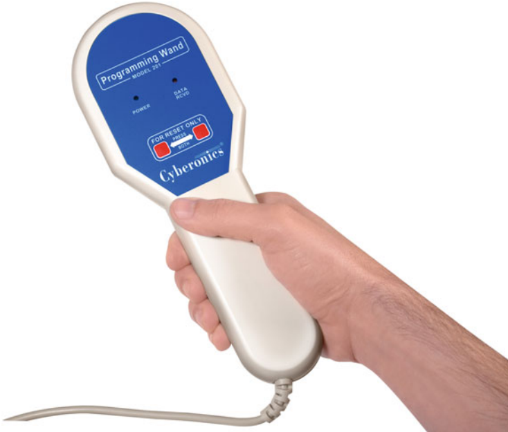
Fig. 4 The VNS device programming wand. This instrument is held against the skin directly over the implanted VNS generator. The wand is attached to a handheld computer, similar to a smartphone, which allows for modification of electrical parameters changes and is used for assessments of circuit integrity (successful transmission of current to the vagus nerve), as well as programming the electrical parameters being delivered during VNS. Source: Reproduced with permission of LivaNova
